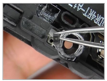
There is a small, black plastic spacer underneath the metal bracket at the upper screw. The upper screw goes through the metal bracket then through this plastic spacer.
