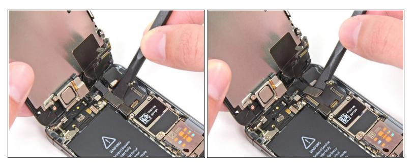
• Finally, disconnect the digitizer cable connector.
