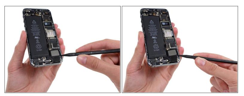
Use the point of a spudger to gently pry between the speaker and the rear case, lifting the speaker enough to grab with your fingers.
