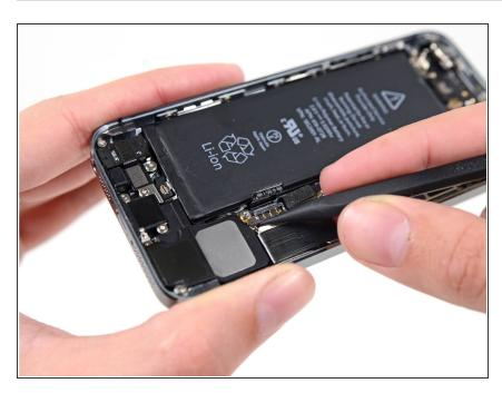
Use the tip of a spudger to pry the antenna cable up from its socket on the logic board.
