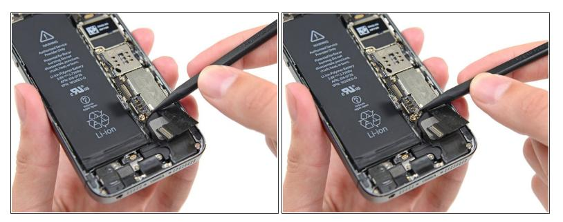
Use the tip of a spudger to pry the antenna cable up from its socket on the logic board.
