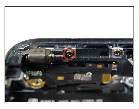
Remove the 1.7 mm Phillips #000 screw securing the vibrator to the rear case.
