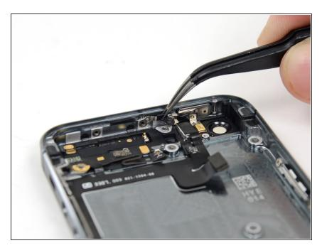
Remove the logic board antenna bracket.
