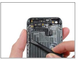
Run the flat end of the spudger under the portion of the cable near the volume control buttons.
