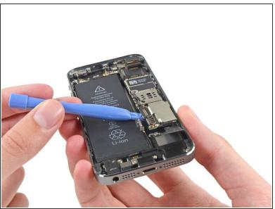
Use a plastic opening tool to lift the logic board up enough to grab with your fingers.
