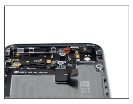
Remove the 2.1 mm Phillips #000 screw securing the contact clip and power/sleep button bracket.
