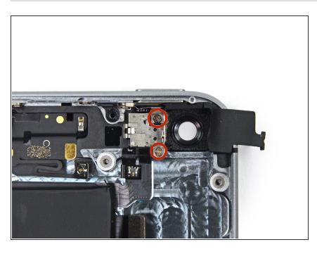
Remove the two 1.6 mm Phillips #000 screws securing the rearfacing camera bracket.
