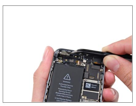
Use a set of tweezers to remove the vibrator from the rear case. To reassemble your device, follow these instructions in reverse order.
