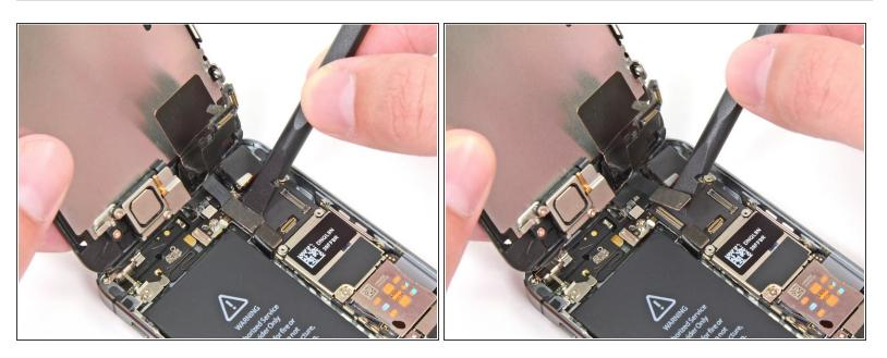
• Finally, disconnect the digitizer cable connector.
