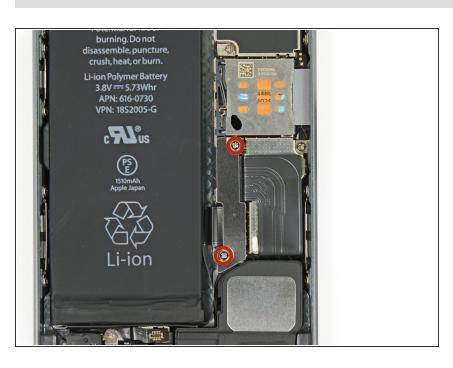
Remove the two 1.6 mm Phillips #000 screws securing the metal battery connector bracket to the logic board.
