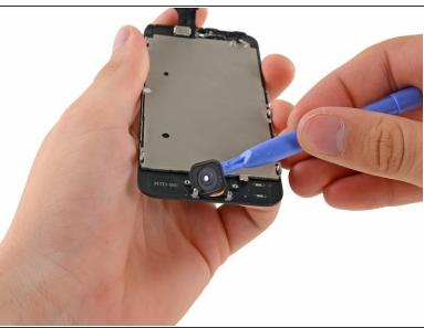
Use a plastic opening tool to pry the home button up from the display assembly.
