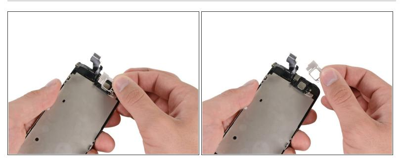
Remove the earpiece speaker bracket from the display assembly.
