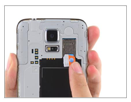
• Repeat the above procedure to remove the SIM card.
