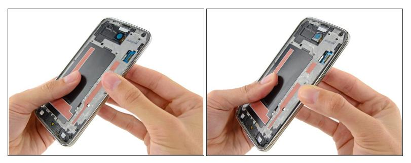
Continue on to the right side of the silver bezel, pulling away from the interior section of the midframe to separate the two halves.
