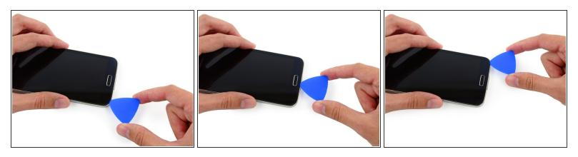
The bottom end of the phone contains the soft button and home button ribbon cables. If you insert the opening pick too far into the phone you risk cutting these cables.
