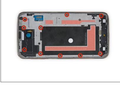
Remove the ten 3.4 mm Phillips #000 screws from the display side of the midframe.
