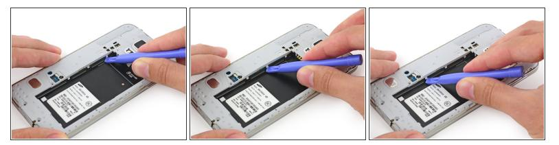
Gently run a plastic opening tool down along the left inner side of the interior frame to separate the three white plastic clips.
