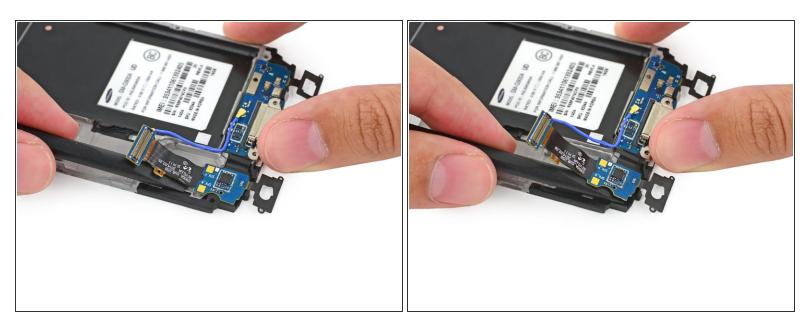
• Gently slide the flat end of a spudger in between the daughterboard cable and the interior midframe to begin to separate the adhesive holding it down.
