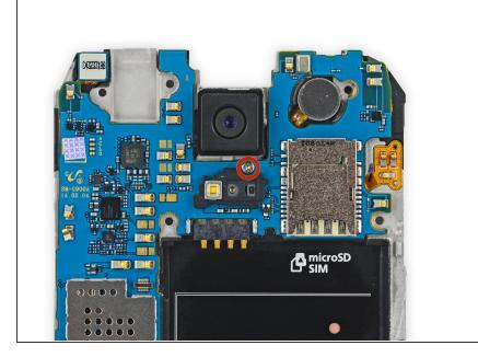
Remove the single 3.0 mm Phillips #000 screw securing the motherboard to the midframe.
