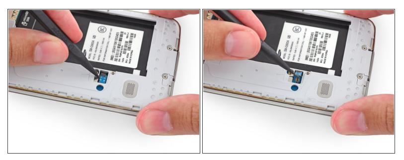
• Use the sharp tip of a spudger to pry the home button cable connector straight up off its socket.
