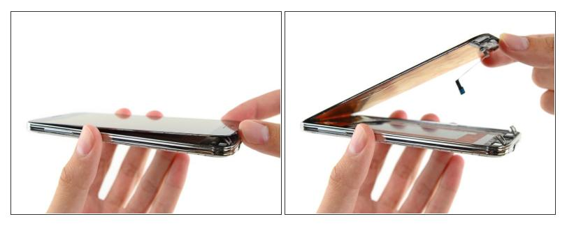
• Slightly lift, but do **not** remove, the home button end of display assembly.
