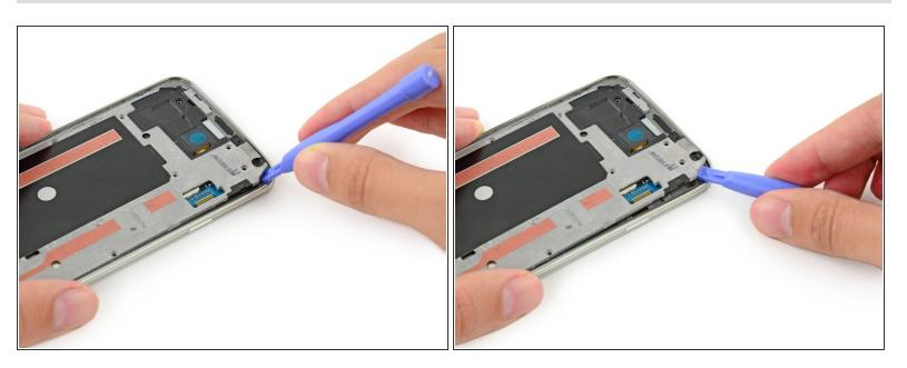
Use a plastic opening tool to pry any remaining corners out of the silver bezel.
