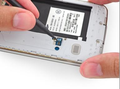
• Use the sharp tip of a spudger to pry the home button cable connector straight up off its socket.
