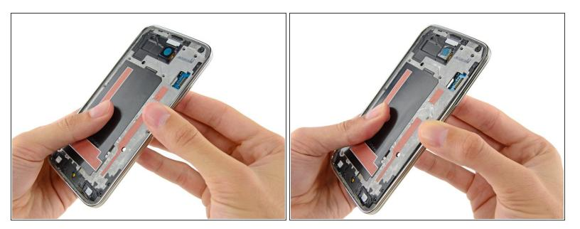
Continue on to the right side of the silver bezel, pulling away from the interior section of the midframe to separate the two halves.
