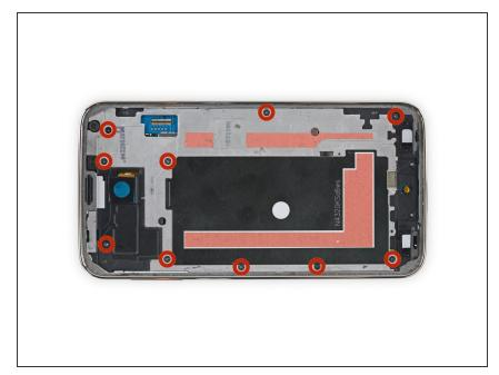
Remove the ten 3.4 mm Phillips #000 screws from the display side of the midframe.
