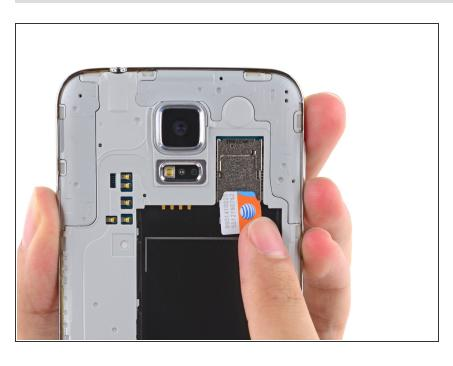
Repeat the above procedure to remove the SIM card. To reassemble your device, follow these instructions in reverse order.
