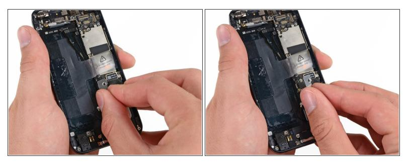
• Remove the mid-section bracket from the logic board.
