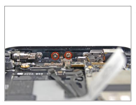
Remove the two 1.3 mm Phillips screws from the inner top of the rear case.
