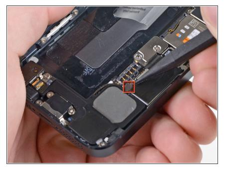
Use the tip of a spudger to pry the cellular data antenna cable connector up from its socket on the logic board, just above the speaker enclosure.
