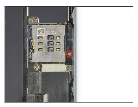
Remove the 2.1 mm Phillips #00 securing the SIM eject lever.
