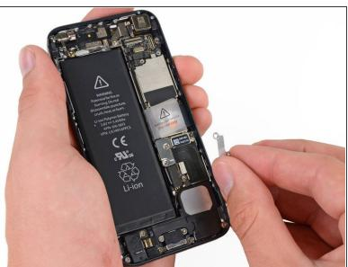
Remove the metal bracket securing the battery connector from the iPhone.
