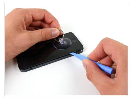
Continue to pry up around the sides of the front panel assembly, detaching the clips along the left and right side.
