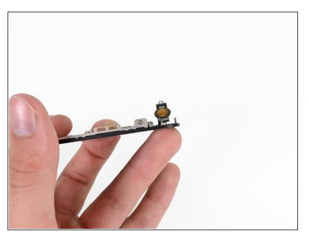
Gently press up on the center of the home button from the display side of the display assembly, to loosen the
