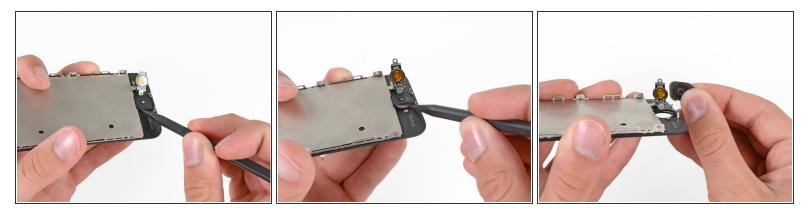
• Once the home button has started to separate from the display assembly, use the tip of a spudger to completely lift the button from the adhesive securing it.
