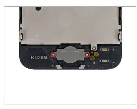
Remove the two 1.3 mm Phillips screws securing the home button bracket to the display assembly.
